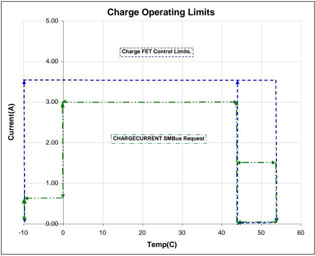
NOTE: If not charging & temperature > 45C then the battery enters Charge-Inhibit where ChargingCurrent() = 0 until temperature  $\leq$  44C.
