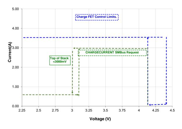
NOTE: The charging current requested from 3.0 to 4.2 V is defined by the temperature of the pack as shown in the preceding charge operating limits graph in this section. A 3.0A charge current is shown in this graph to represent the current defined by said graph.
