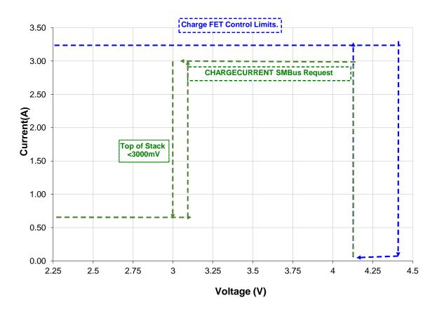
NOTE: The charging current requested from 3.0 to 4.2 V is defined by the temperature of the pack as shown in the preceding charge operating limits graph in this section. A 3A charge current is shown in this graph to represent the current defined by said graph.
